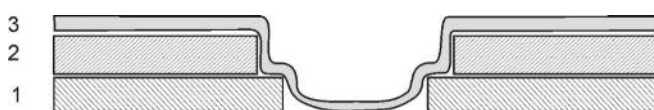
FIG. 3. LOCATION OF THE TWO PARTS OF THE MOULD (1, 2) AND THE MOULDED MATERIAL (3) IN BRAILLE MANUFACTURING PROCESS BY THE ADVANCED VACUUM FORMING METHOD (OUR OWN DESIGN)
