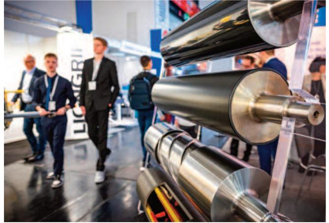
constant and homogeneous surface temperature distribution, as this is the prerequisite for uniform web tempering.
