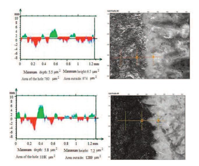
FIG.6. PROFILE OF THE AREA OF OVERPRINT (1A AND 1 B) AND TOPOGRAPHY OF SURFACE (2A AND 2 B) AT THE MODES OF LASER MARKING: A): P=12 W, V=240 MM/S; B): P=14 W, V=240 MM/S.
