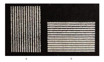
FIG.3. SAMPLE OF LINE OF LASER MARKING, THICKNESS OF 1 POINT IN LONGITUDINAL (A) AND TRANSVERSE (B) DIRECTION ON THE SURFACE OF CARDBOARD COPY, PRINTED WITH BLACK OFFSET INK and larger focusing. The shorter focal length means smaller marking area and narrower sharpness.
