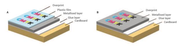
FIG. 1. COMPARISON OF THE STRUCTURE OF PRINTED LAMINATES WITH TRADITIONAL METALLISED FOIL (A) AND TRANSFERABLE FILM (B)
