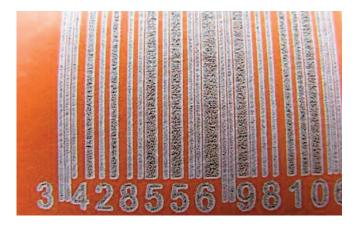
FIG.5. EXAMPLE OF BAR CODE ON CARDBOARD GC-2 (MODES OF LASER MARKING: POWER P=14 W, RATE V=240 MM/S)
