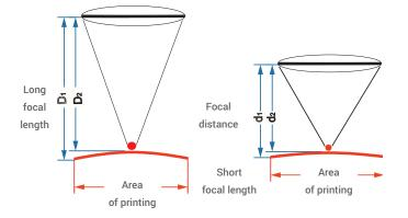
FIG.2. CALCULATION OF FOCAL LENGTH DURING LASER MARKING
