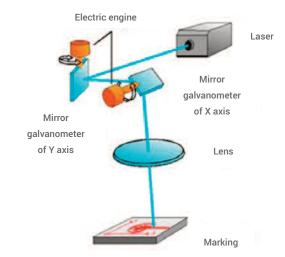
FIG.1. SCHEME OF MARKING WITH CO2 LASER [5]
