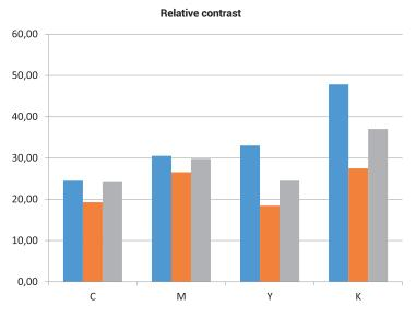
FIG. 3. RELATIVE CONTRAST FOR PARTICULAR MATERIALS; 📕 HIPS; 📕 PMMA, 📕 PVC
