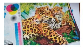
FIG. 5. TEST OBJECTS PRINTED ON A NAPKIN TO DETERMINE DENSITOMETRIC INDICATORS
