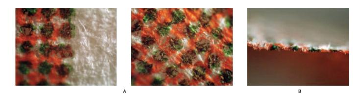
FIG. 6. MICROPHOTOGRAPH OF THE SURFACE (A) AND CROSS-SECTION (B) OF THE PRINTED IMAGE ON A NAPKIN (MAGNIFIED ×200 TIME)
